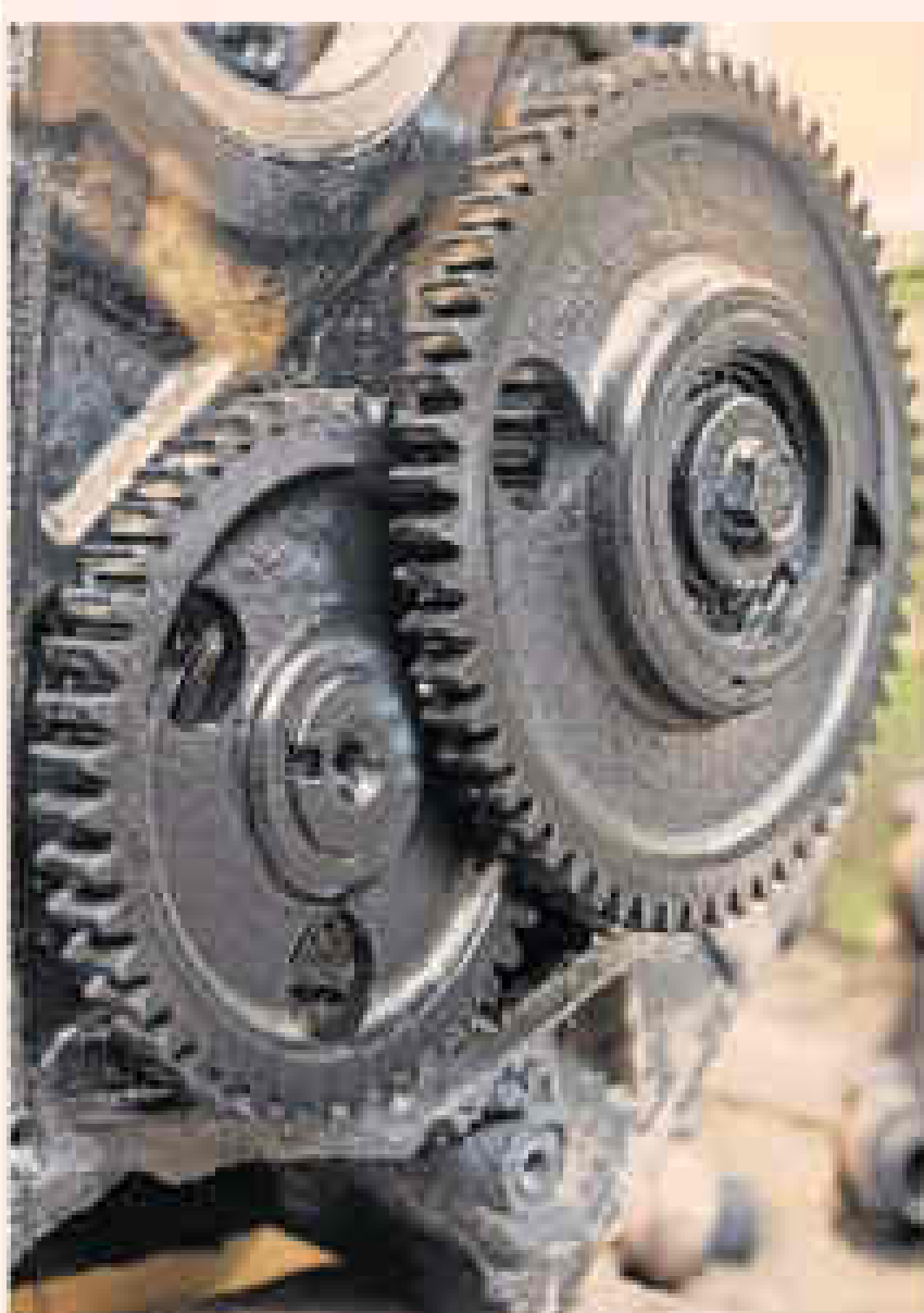
Gears with prime numbers of teeth ensure wear is evenly distributed
